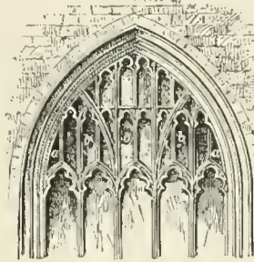
Head of Perpendicular Window. b, b, b, batment-lights; a, a, angel-lights.
